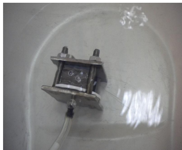
Fig. 5. Determination of the maximum pore sizes on a standard filter element (a) and EO FMTS (b)
