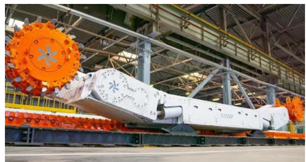
Fig. 1. The UKD200-500 coal shearer.
