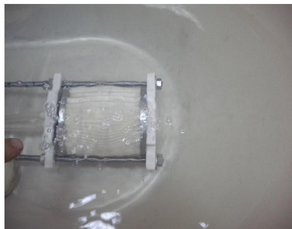
Fig. 4. Tooling assembly with EO FMTS
