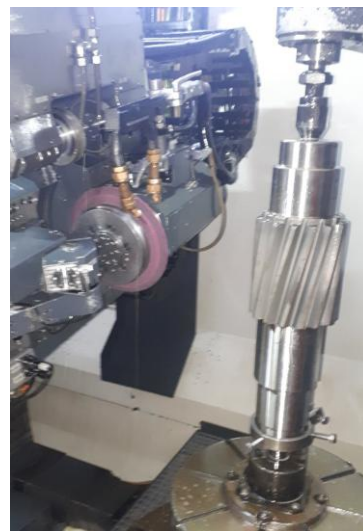
Fig. 9. Installation of a chrome corundum grinding wheel on the machine.
